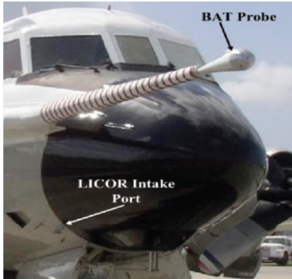
FIG. 3. Location of the BAT turbulence probe and LI-COR fast-response humidity probe on the WP-3D aircraft.
